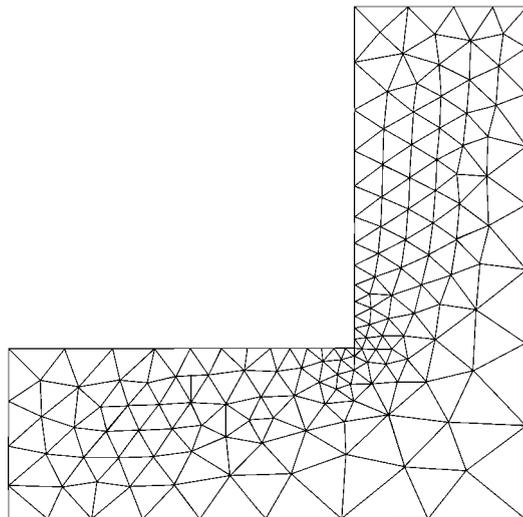
Fig. 2. Mesh used for the perforated plate: imposed loading.
