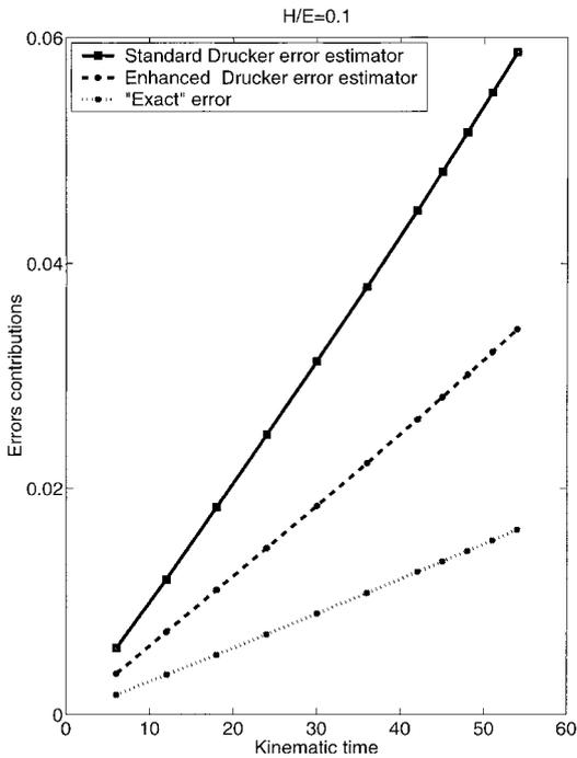
Fig. 4. Contributions to the error for a plastic slope of 0.1.
