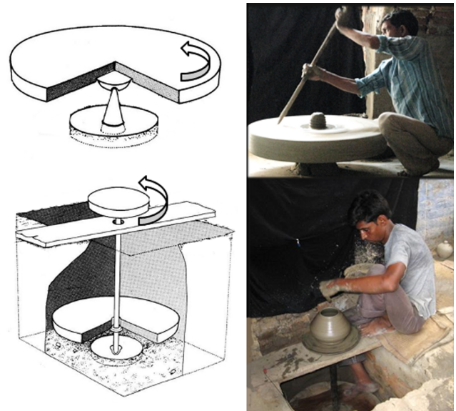
Fig. 2. The two common wheels used in northern India. Top panel: the high inertia stick-wheel used by the Prajapati potters. Bottom panel: the low-inertia kick-wheel used by the Multani potters. Drawings are adapted from Orton et al. (1993). The two wheels evoke distinct body positions: for the stick-wheel potters typically squat (sometimes they use a low stool), while for the kick-wheel potters sit, one leg folded, on a wooden plank.
